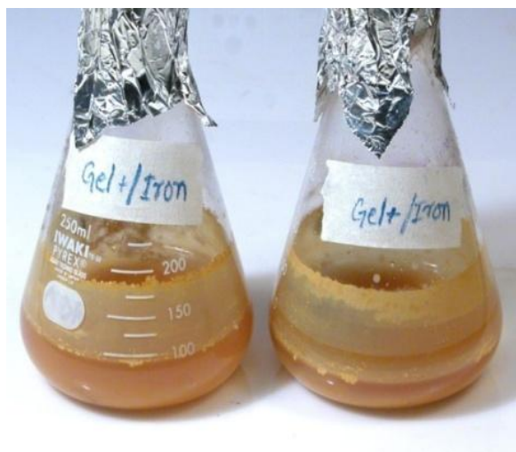
Fig. 3. Conversion of Fe^{2+} into Fe^{3+} by Acidithiobacillus ferrooxidans at 300C, 150 rpm.
