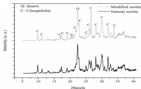
**Fig. 1.** XRD patterns of the Mg-modified and natural zeolites.
