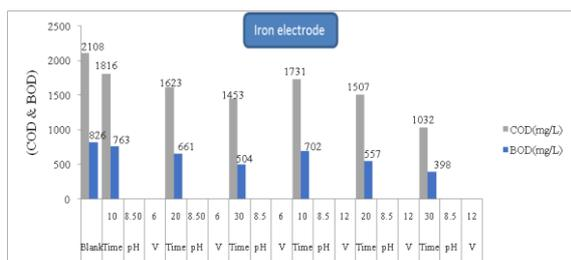
**Fig. 5.** COD and BOD trend of change in alkaline pH using electrochemical method.
