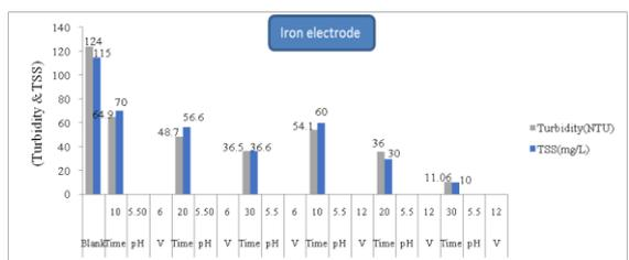
**Fig. 4.** Turbidity and TSS trend of change in acidic pH using electrochemical method.
