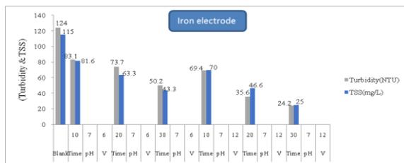
**Fig. 2.** Turbidity and TSS trend of change in pH=7 using electrochemical method.
