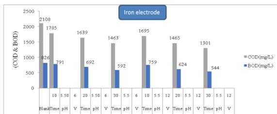
**Fig. 3.** COD and BOD trend of change in acidic pH using electrochemical method.
