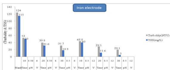
**Fig. 6.** Turbidity and TSS trend of change in alkaline pH using electrochemical method.
