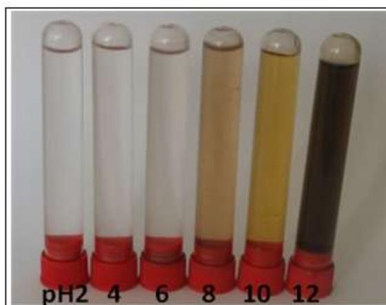
**Fig. 7.** Colors of Ag nanoparticles solution at pH 2, 4, 6, 8, 10, 12.
