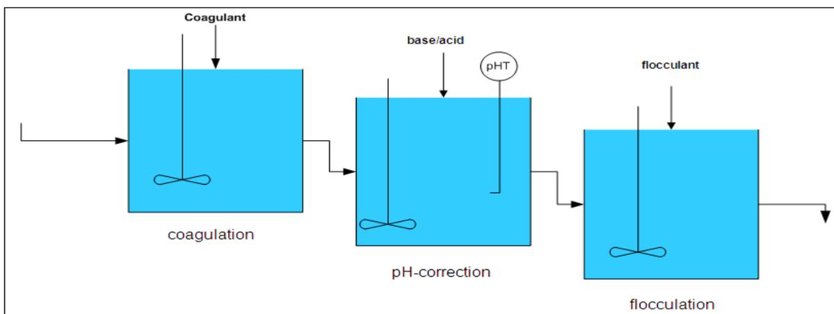
Fig. 2. Components of conventional physico-chemical treatment.
