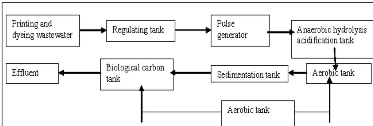
Fig. 11. Anaerobic-aerobic-biological carbon contacts process flow diagram.
