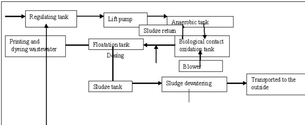
Fig. 10. Hydrolytic acidification-contact oxidation-air floatation process flow diagram.
