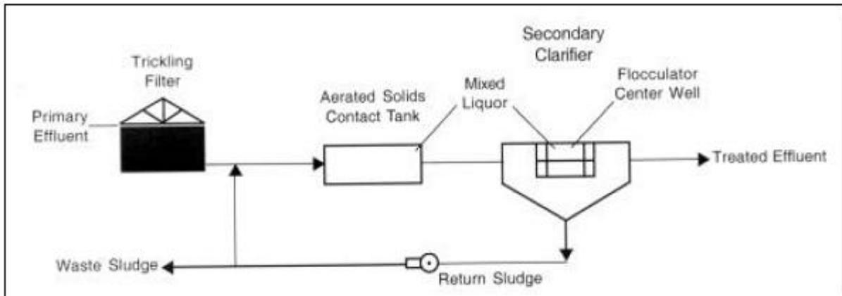
Fig. 4. Secondary treatment Processes.
