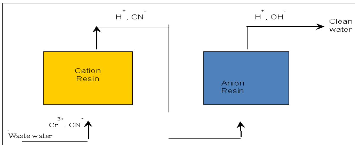
Fig. 8. A Flow diagram of Ion Exchanger.
