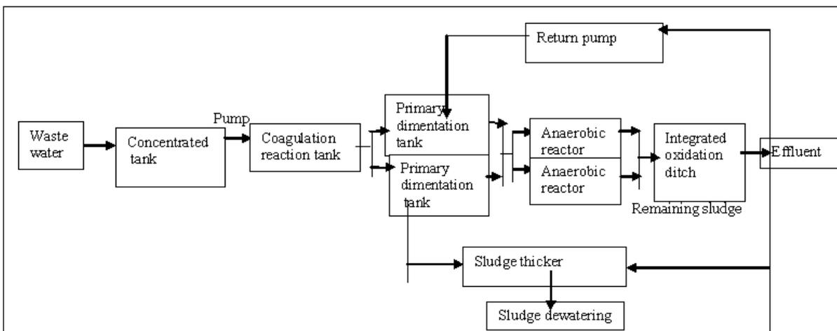
Fig. 12. Coagulation-ABR-oxidation ditch process flow diagram.
