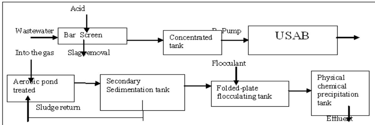
Fig. 13. UASB-aerobic-physicochemical treatment process flow diagram.
