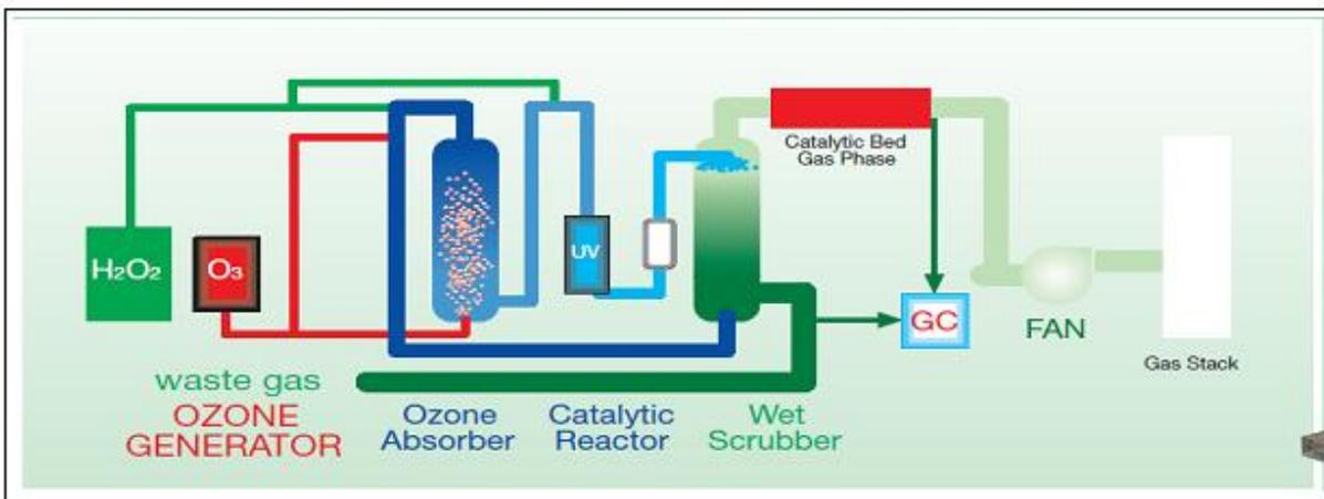
Fig. 14. Advanced Oxidation Processes (AOPs) flow diagram.
