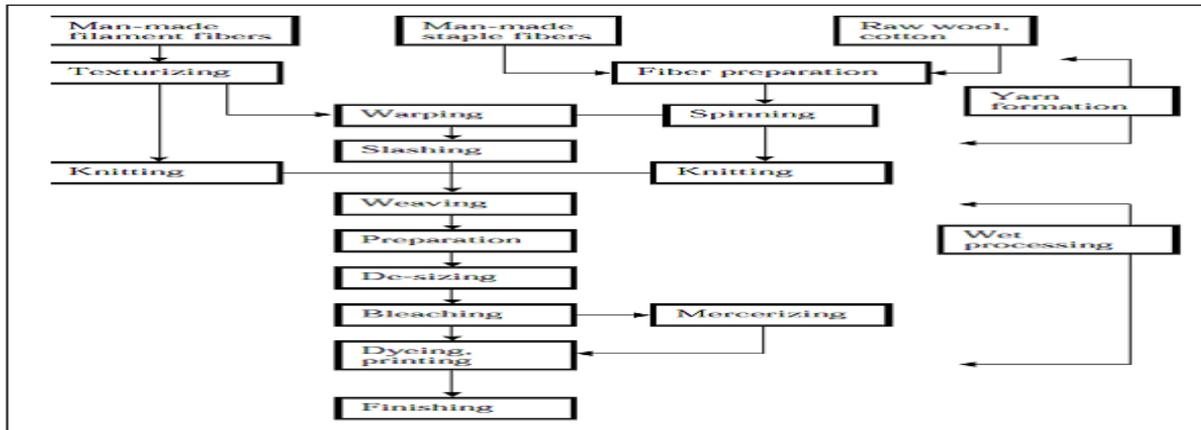
Fig. 1. A flow diagram for various steps involved in processing textile in a cotton mills.
