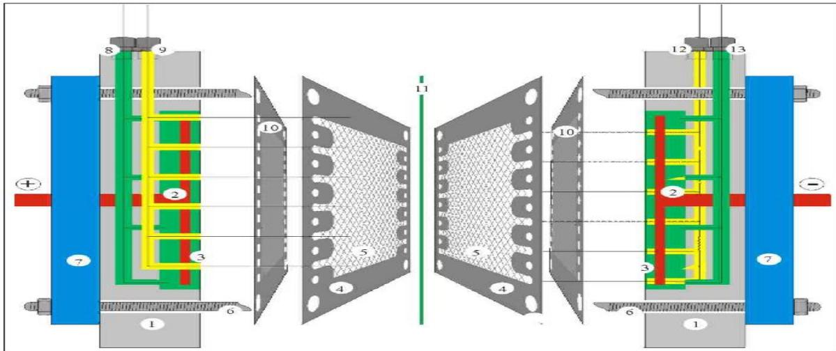
Fig. 7. A typical Electrodeionization (ED) flow diagram.
