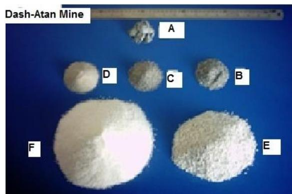
**Fig. 6.** Samples of raw and expanded perlites from DatashAtan Mine (a: aggregate perlite; b: raw perlite with size of 2mm, c: raw perlite with size of 4.1mm, d; raw perlite with size of 0-5.1mm, e:expanded perlite with size of 2.5mm, f: expanded perlite with size of 1.5mm).
