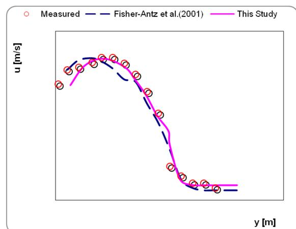
**Fig. 1.** Comparing the results of numerical simulations with actual observations and conclusions in this paper (Fisher Antz *et al.*, 2001) in spite of the composite section vegetation Drdby 0/057.
