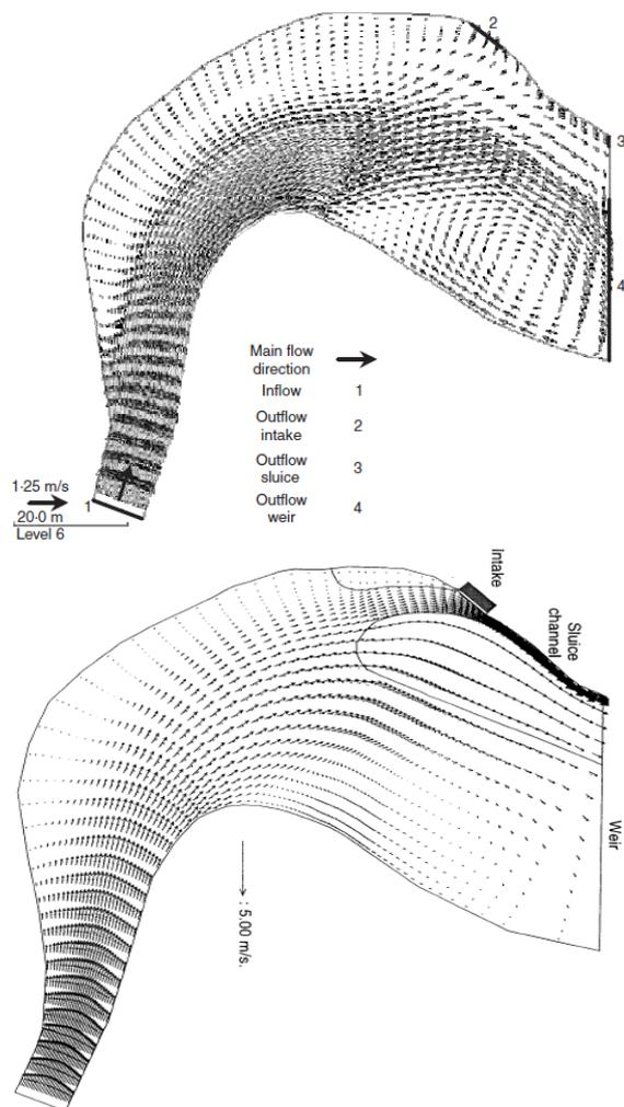
**Fig. 7.** Calculated flow field in PHONICS model in the research (Ruther, 2006).
