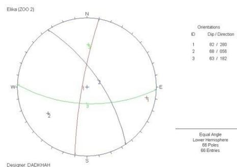
**Fig. 8.** Stereography of discontinuities existing in Elika formation of Zou 2 mine.
