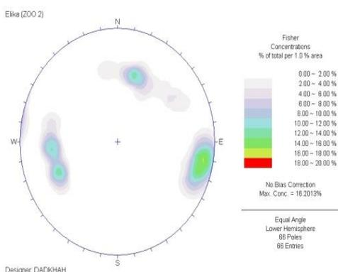
**Fig. 6.** Stereography picture of existed discontinuities in Elika formation Zou 2 mine.
