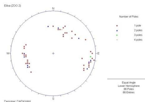
**Fig. 9.** Stereography of polra spots of discontinuities existing in Elika formation of Zou 2 mine.
