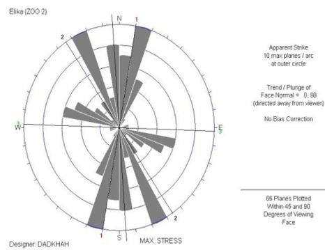
**Fig. 7.** Rose diagram of discontinuities existing in Elika formation of Zou 2 mine.
