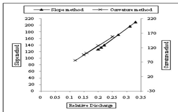
**Fig. 12.** Comparison between slope and curvature method for  $Q_{EF}$  assessment.
