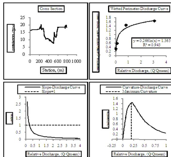
Fig. 8. Cross section, Wetted perimeter-Discharge Graph, Curvature and Slope of wetted perimeter relationship for the fourth section.
