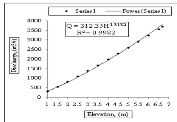
**Fig. 3.** Rating curve graph of Ahwaz Station.
