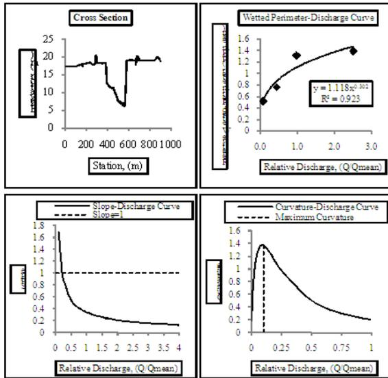
**Fig. 9.** Cross section, Wetted perimeter-Discharge Graph, Curvature and Slope of wetted perimeter relationship for the fifth section.
