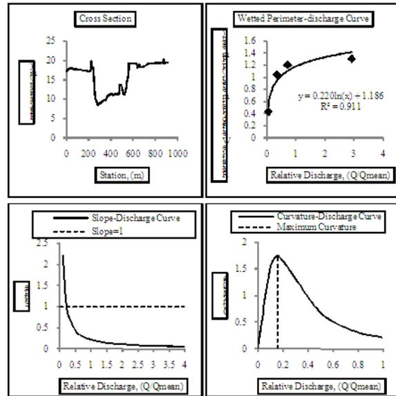
Fig. 7. Cross section, Wetted perimeter-Discharge Graph, Curvature and Slope of wetted perimeter relationship for the third section.
