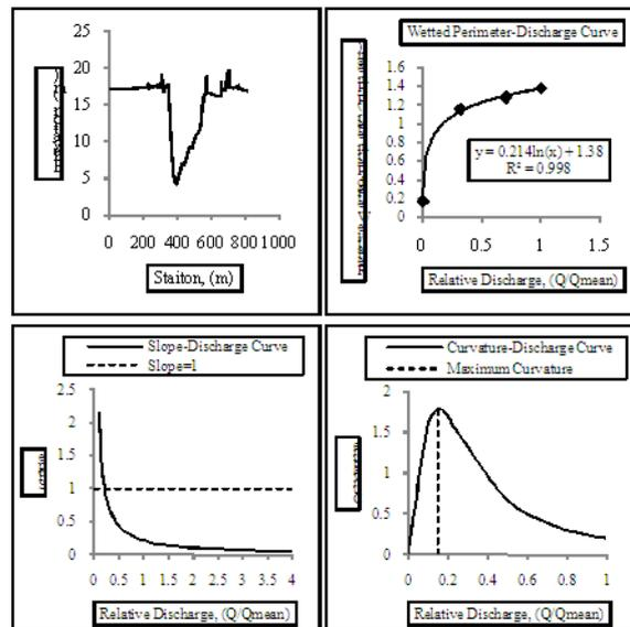
**Fig. 11.** Cross section, Wetted perimeter-Discharge Graph, Curvature and Slope of wetted perimeter relationship for the seventh section.
