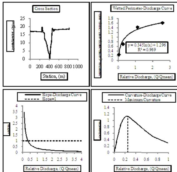
**Fig. 10.** Cross section, Wetted perimeter-Discharge Graph, Curvature and Slope of wetted perimeter relationship for the sixth section.
