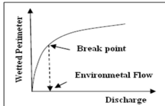
**Fig. 2.** Schematic view of breakpoint wetted perimeter-discharge curve.
