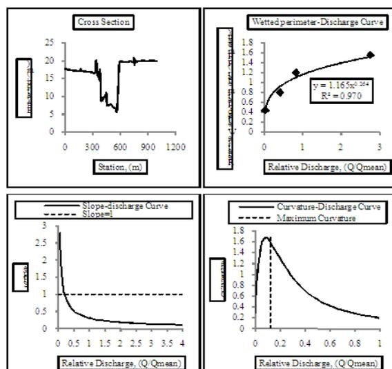
Fig. 6. Cross section, Wetted perimeter-Discharge Graph, Curvature and Slope of wetted perimeter relationship for the second section.
