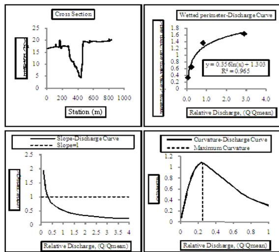
Fig. 5. Cross section, Wetted perimeter-Discharge Graph, Curvature and Slope of wetted perimeter relationship for the first section.
