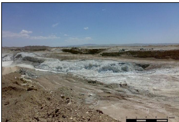
Fig. 7. view of mineral body in the location of profile 11, removal of overburden after resistivity surveying.
