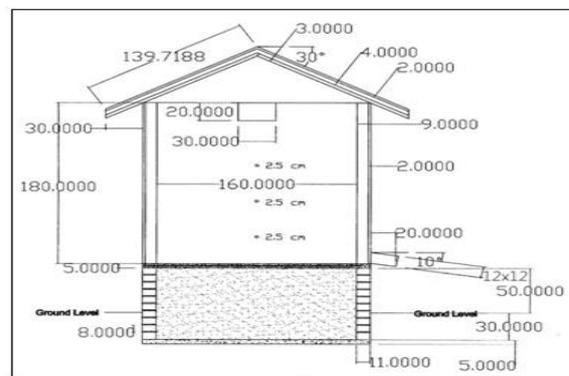
**Fig. 2.** Schematic diagram of the straw-clay bin.
