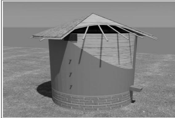
**Fig. 3.** Three dimensional view of the straw-clay bin.
