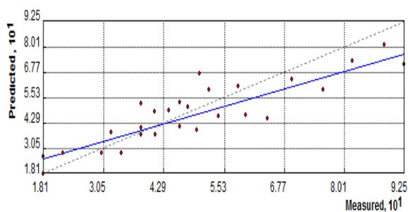
Fig. 3. Scatter plot of estimated and measure values in cokriging interpolation method for soil organic carbon data.
