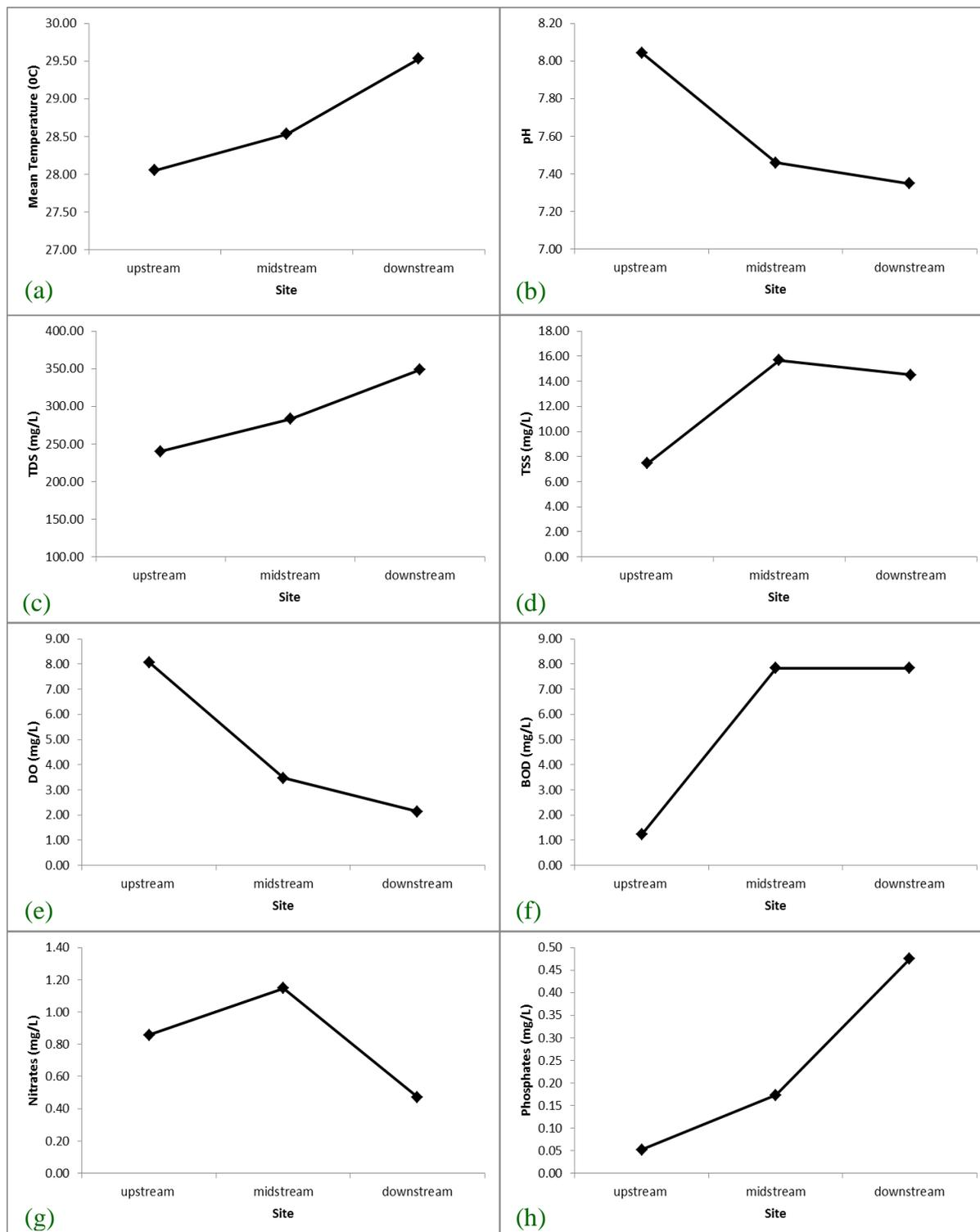
**Fig. 2.** Mean (a) temperature, (b) pH, (c) TDS, (d) TSS, (e) DO, (f) BOD, (g) nitrates and (h) total P of Bulacao River.
