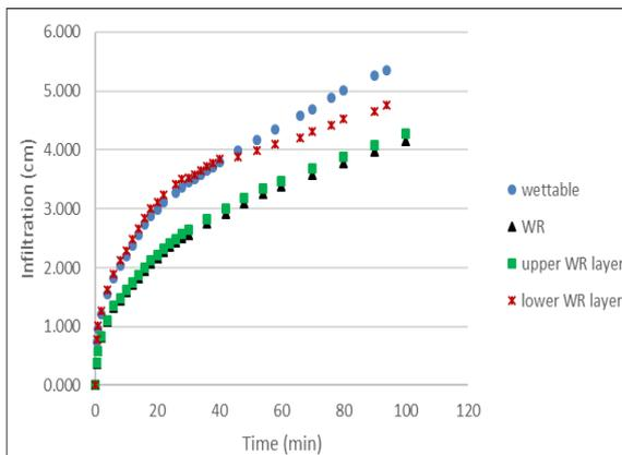
**Fig. 3.** Cumulative infiltration in the clay loam soil.
