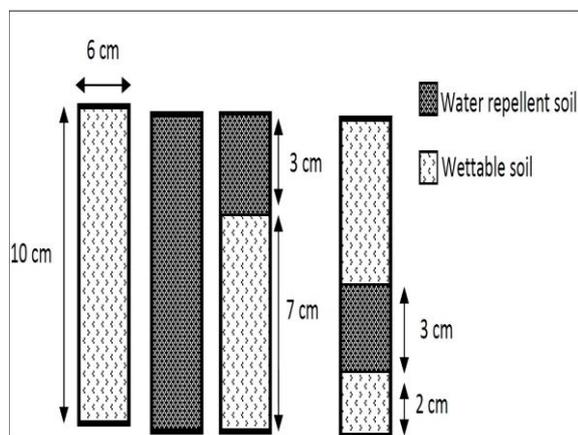
**Fig. 1.** Water repellent layer placement in soil columns.
