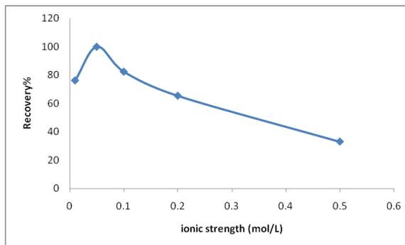
**Fig. 4.** effect of ionic strength on Co (II) extraction.
