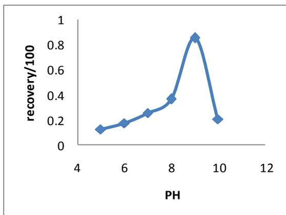
**Fig. 2.** effect of PH on Co (II) extraction.
