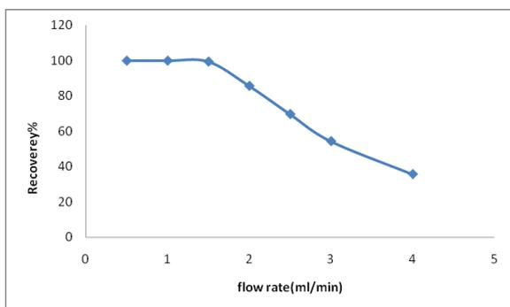
**Fig. 3.** Effect of sample flow rate on extraction process.
