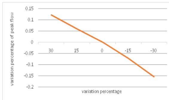
**Fig. 3.** Percentage change in impermeable surfaces and its effect on peak flow in percentage.
