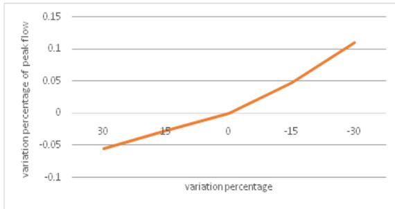
**Fig. 5.** Percentage of Manning roughness coefficient impermeable areas and its impact on peak flow in percentage.
