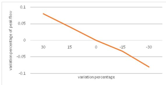
**Fig. 6.** The percentage change in the equivalent rectangle width and its impact on peak flow in percentage.
