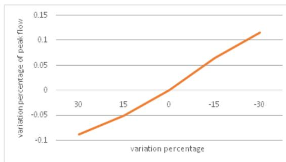
**Fig. 4.** Percentage of channel roughness coefficient of variation and its impact on peak flow in percentage.
