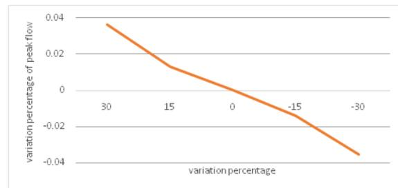
**Fig. 7.** Percentage of slope change and its impact on peak flow in percentage
