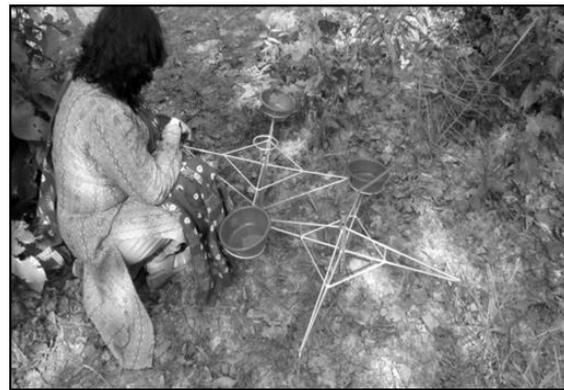
**Fig. 4.** Dismantled parts of the unique adjustable bee trap
