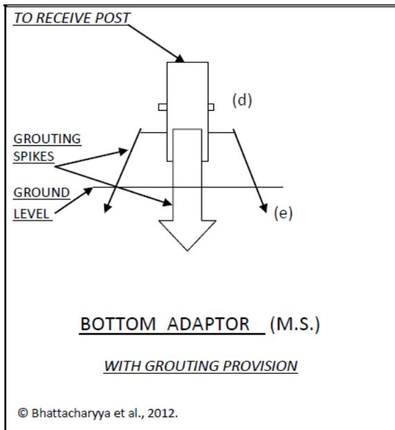
**Fig. 2.** Elevation of bottom grouting part of the adjustable trap (For labels see text)
