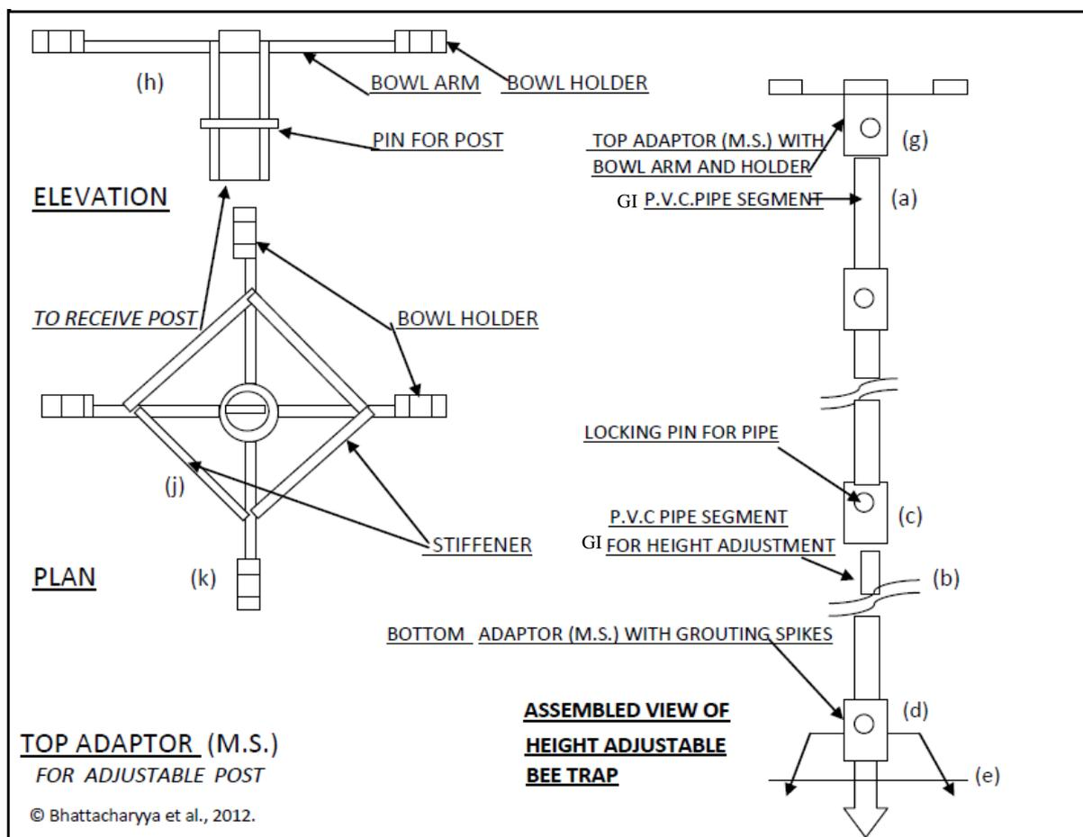
**Fig. 1.** Lateral view of the assembled trap (on the right) and separate plan and elevation of the top display/baiting part (on the left). For labels, see text.
