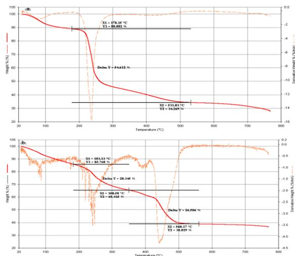
**Fig. 2.** TGA of crude Chitosan (a) and Chitosan-g-PolyAN (b).
