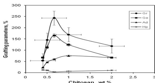
**Fig. 6.** Effect of polysaccharide concentration on the grafting parameters.
