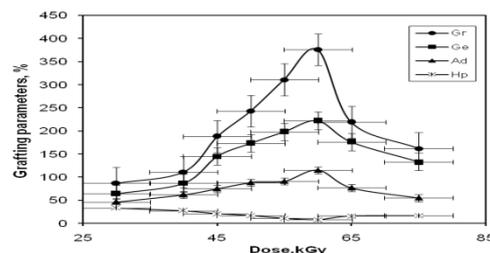
**Fig. 5.** Grafting parameters as functions of doses of δ-rays.
