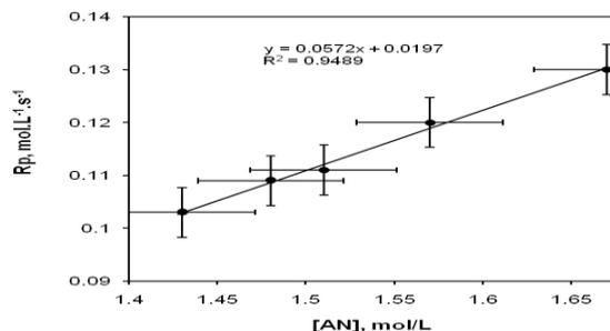
**Fig. 3.** Plot of Rp versus monomer concentration.
