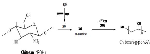
**Scheme 1.** A brief proposed mechanism for  $\gamma$ -rays-induced grafting of poly(AN) onto Chitosan.
