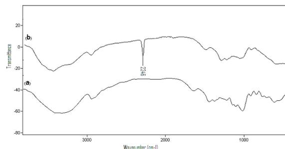
**Fig. 1.** FTIR spectra of (a) crude Chitosan and (b) homopolymer-free Chitosan -g-PolyAN.
