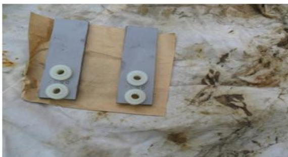
**Fig. 1.** Coupons before insertion into oil pipelines.
