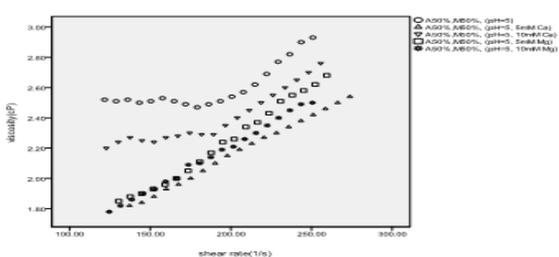
**Fig. 11.** Viscosity as a function of shear rate of sodium alginate - HPC (75/25) solution at A(pH 3), B(5) and C(pH=7) without or with salts.
