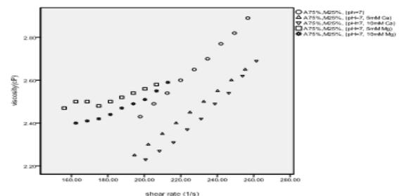
**Fig. 9.** Viscosity as a function of shear rate of sodium alginate - HPC (75/25) solution at A(pH 3), B(5) and C(pH=7) without or with salts.
