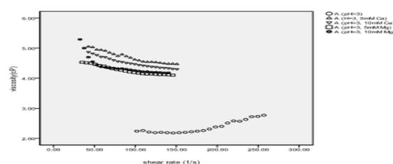
**Fig. 2.** Viscosity as a function of shear rate of methylcellulose solution at A(pH 3), B(5) and C(pH=7) without or with salts.
