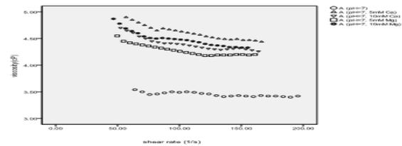
**Fig. 3.** Viscosity as a function of shear rate of methylcellulose solution at A(pH 3), B(5) and C(pH=7) without or with salts.
