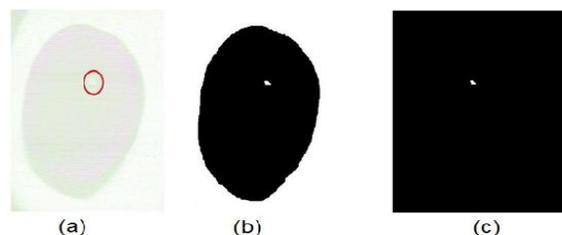
**Fig. 2.** from left to right: a) UV image from the camera; b) image binarization and separation of the apple sample; and c) binarization and separation of the bruised area.
