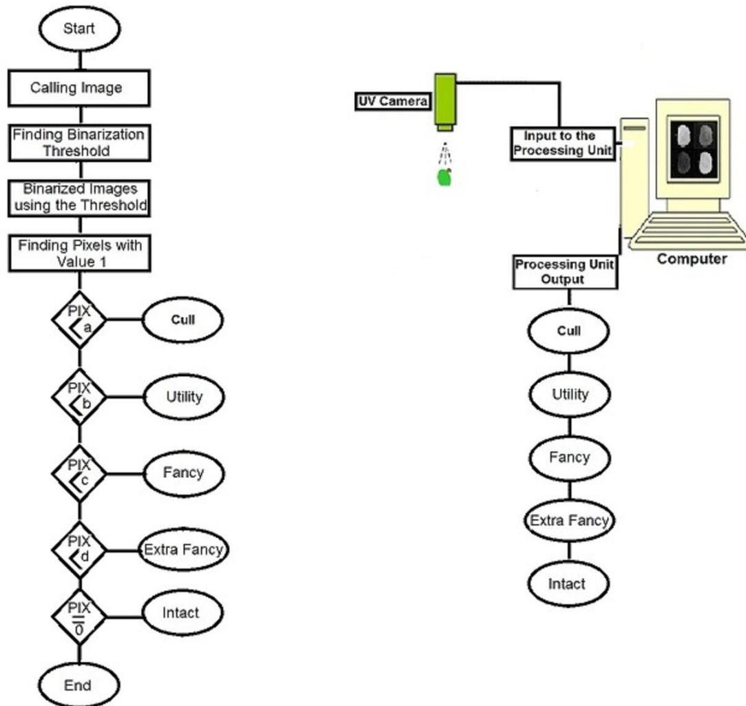
**Fig. 1.** schematic view of the grading process (left) and the imaging and image processing (right).
