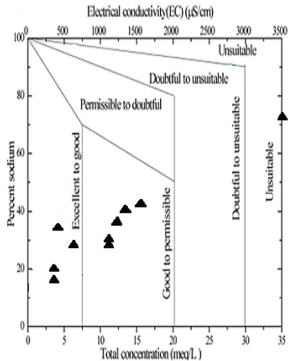
**Fig. 5.** U.S. Diagram for classification of salinity and alkalinity hazards.
