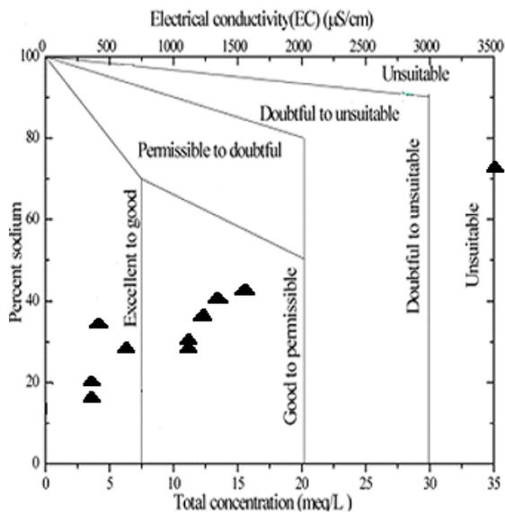
**Fig. 4.** Wilcox Diagram for plot sodium percent versus electrical conductance.
