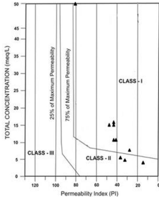
**Fig. 6.** Classification of irrigation water based on the permeability index.
