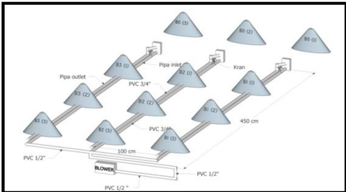
**Fig. 1.** Aerated static piles design.
