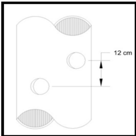
**Fig. 2.** Perforated Polyvinyl Chloride (PVC) pipes.
