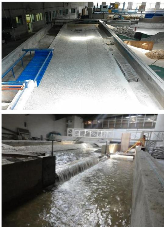
**Fig. 5.** Images from the side weir and channel of the studied.
