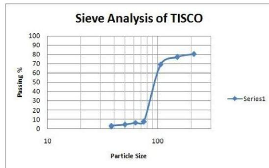
**Fig.5c.** Sieve analysis of TISCO Jamadoba fly ash.
