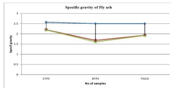
**Fig.2.** Specific gravity of fly ash.
