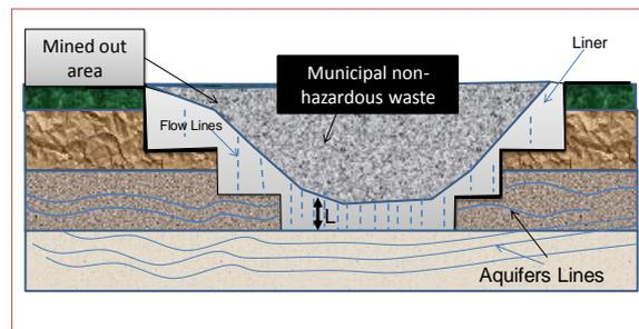
**Fig. 1.** Proposed design of Landfill liner for mined out areas of Jharia coalfield.
