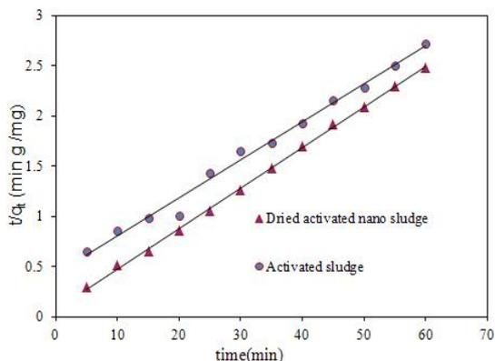
**Fig. 7.** kinetic experimental data and pseudo-second -order model for Cu (II) biosorption by DAS and DANS.
