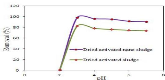
**Fig.2.** The influence of initial pH on the removal efficiency of Cu(II) by (DAS) and (DANS) (C<sub>0</sub> 25mg/L, temperature 25 °C and biomass dosage 1g/L).
