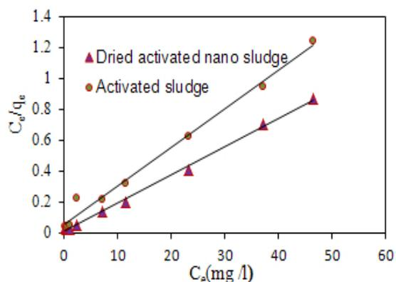
**Fig. 6.** Langmuir isotherms for the adsorption of copper by DAS and DANDS ( $C_0$  25 mg /L, temperature 25°C, biomass dosage 1g/L and pH: 3).
