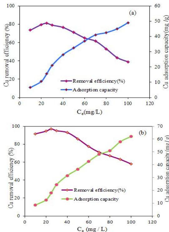
**Fig. 3.** Effect of initial Cu (II) concentration on copper removal efficiency by (a) DAS and (b) DANS (C<sub>0</sub> 25mg/L, temperature 25 °C, biomass dosage 1g/L and pH 3).
