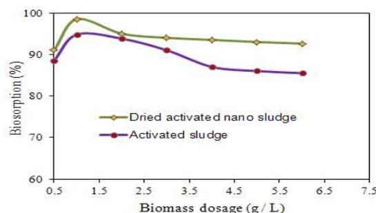
**Fig. 5.** Effect of biomass amount (g) on copper removal efficiency by DAS and DANS ( $C_0$  25 mg/L, temperature 25°C, biomass dosage 1 g/L and pH 3).
