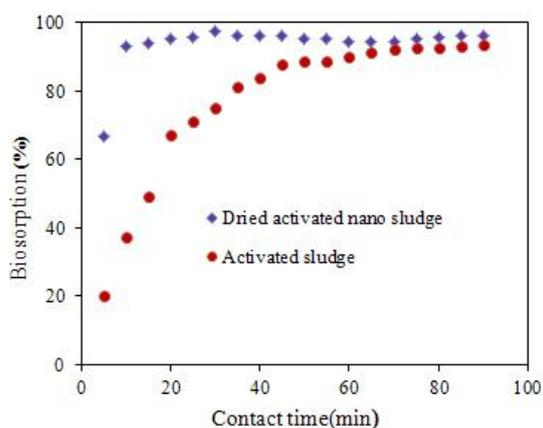
**Fig. 4.** Effect of contact time on copper removal efficiency by DAS and DANS ( $C_0$  25 mg/L, temperature 25 °C, biomass dosage 1 g/L and pH 3).
